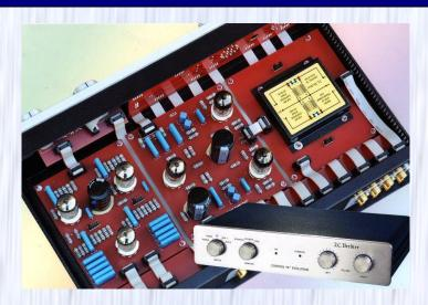
This new preamplifier perpetuates all the values which have established the reputation of the Control "B," adding some refinements in relation to the permanent search for more precise, more stable, more musical components. All circuits are modular. Each printed circuit is dedicated to a unique function. This enables the user to change operating modes or to accommodate different components instantaneously and without adjustment.
